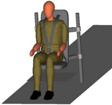
Figure 11: Dummy and Harness System Setup
